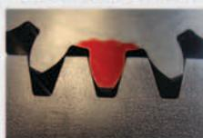
Inside rack & pinion systems, the loads are concentrated on only one tooth
