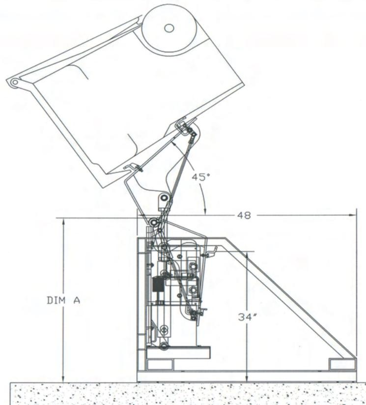
MODEL      DIM A      (CYLINDER-TYPE INDUSTRIAL LIFTERS)
