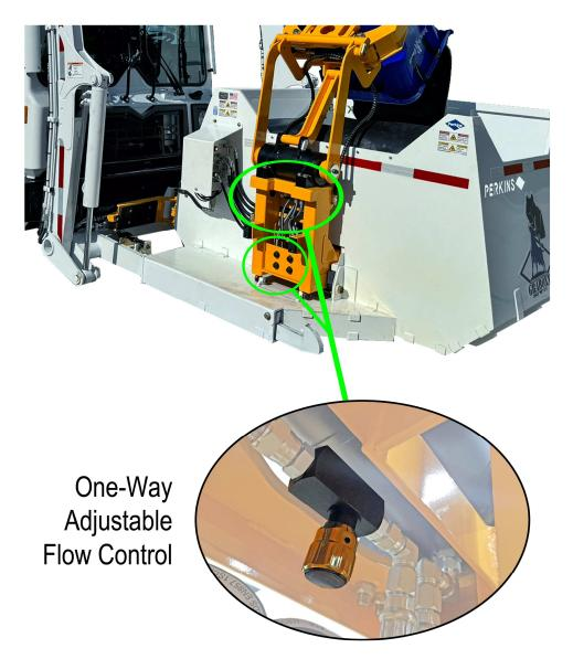
**One Way Adjustable Flow Control**: Located tucked underneath the rotary actuator is a one-way adjustable flow control, which leads to the left-hand port of the actuator. Its function is to slow down the gripper assembly/ actuator when it is rotating down, preventing the cart from slamming back down into the ground. This valve does NOT affect the rotate-up speed.
